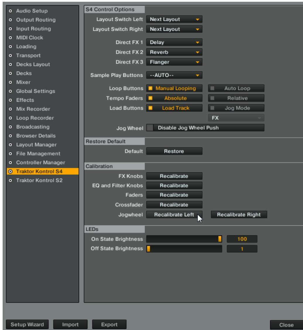
4. The following window presents you with a couple of options. Click [Calibrate](#) to start calibration of the left jog wheel. (The [Restore](#) option lets you restore the calibration settings to the factory settings. Use this option at a later stage if you're unhappy with the outcome of the manual calibration.)
